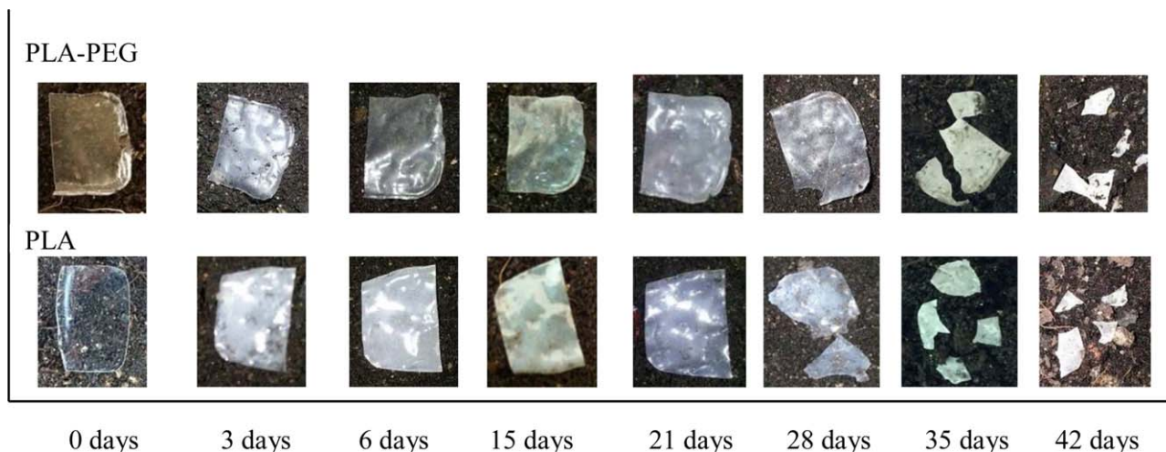
Figure 7. Photographs of neat PLA and PLA-PEG blend at different incubation times at 60 °C. [Color figure can be viewed in the online issue, which is available at wileyonlinelibrary.com .]
